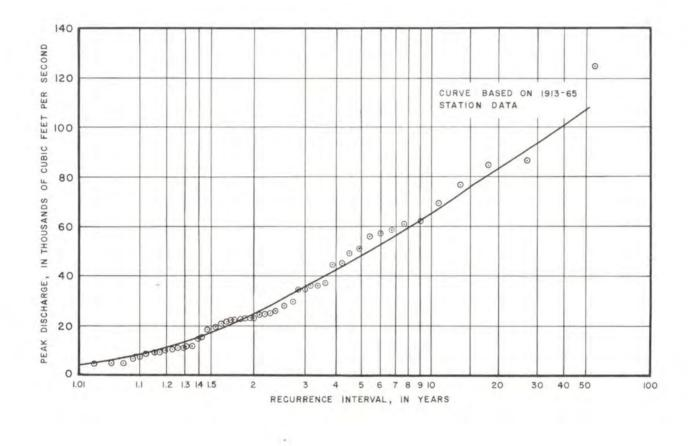
Figure 1. Flood-frequency curve for Current River at Van Buren, Missouri.
