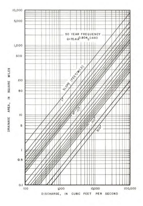
Figure 2f. Graphical solution of the 50-year equation.
