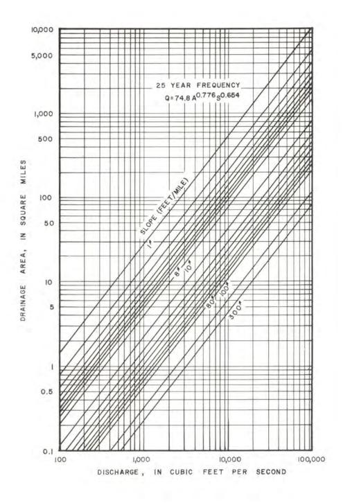
Figure 2e. Graphical solution of the 25-year equation.
