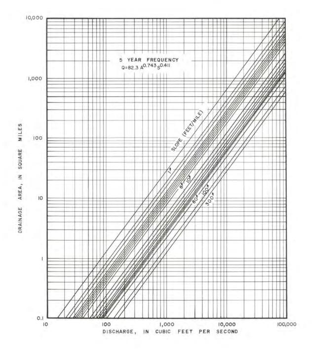
Figure 2c. Graphical solution of the 5-year equation.
