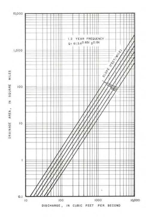
Figure 2a. Graphical solution of 1.2-year equation.
