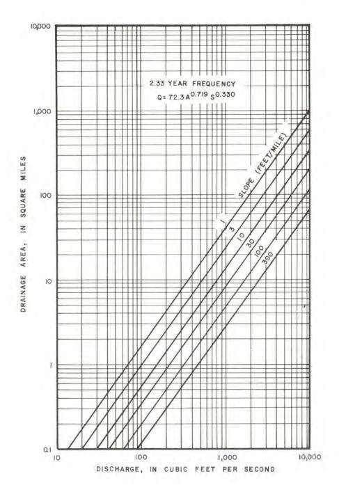
Figure 2b. Graphical solution of the 2.33-year equation.
