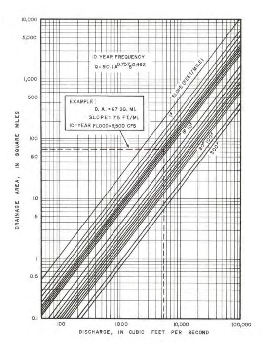
Figure 2d. Graphical solution of the 10-year equation.
