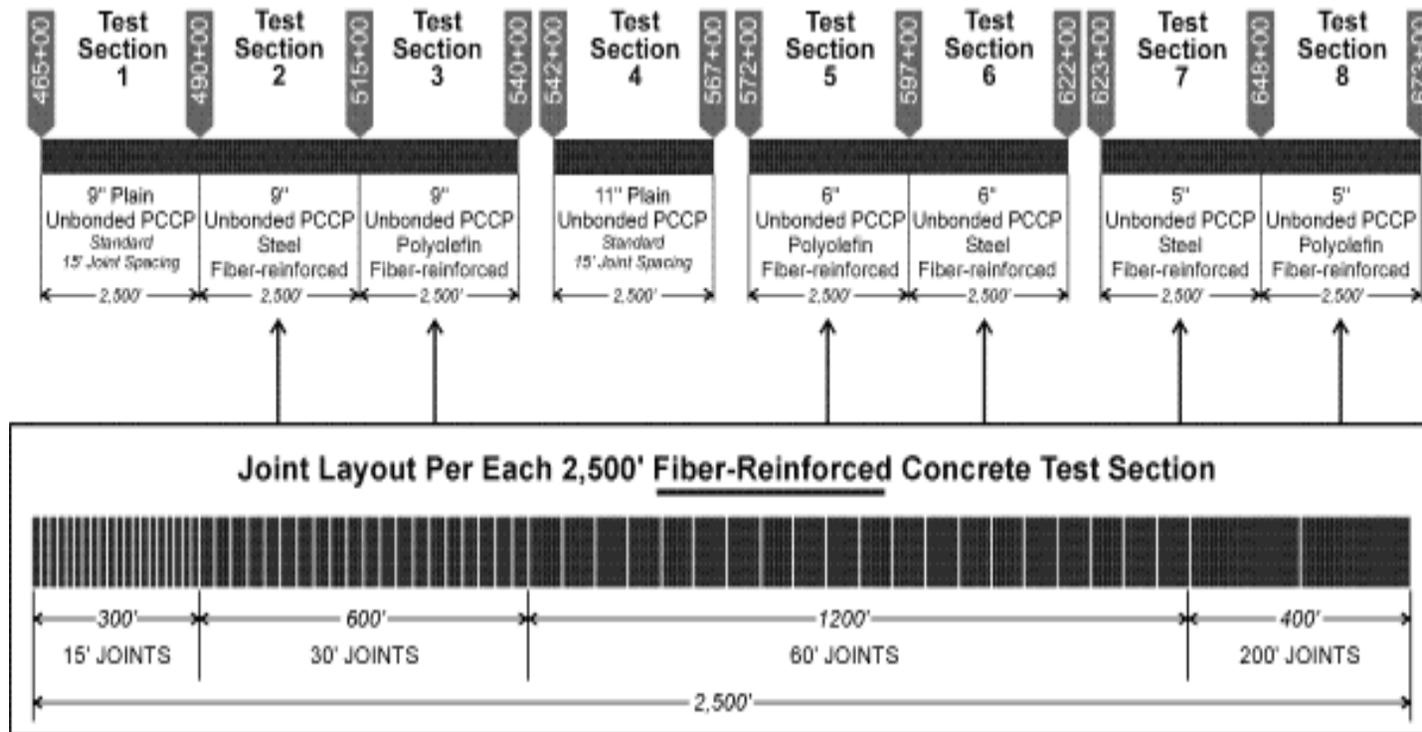
Note: Non-fiber-reinforced concrete test sections and transition areas will have standard 15' joint spacing. Longitudinal joint with tie bars, according to standard, will be placed full length of the unbonded overlay.
