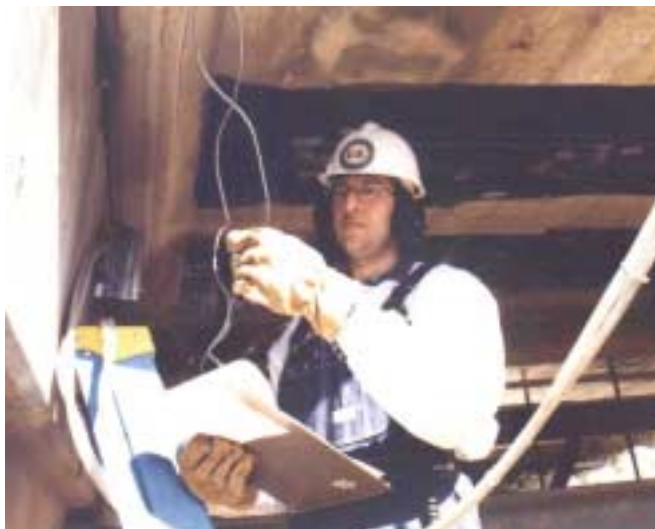
Figure 4.23. Checking the strain gages prior to testing.
