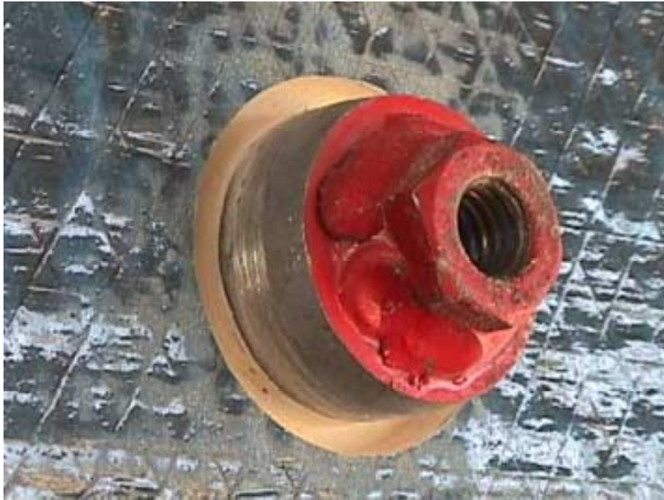
Figure 3.13. Adhesion fixture bonded to the FRP sheet.
