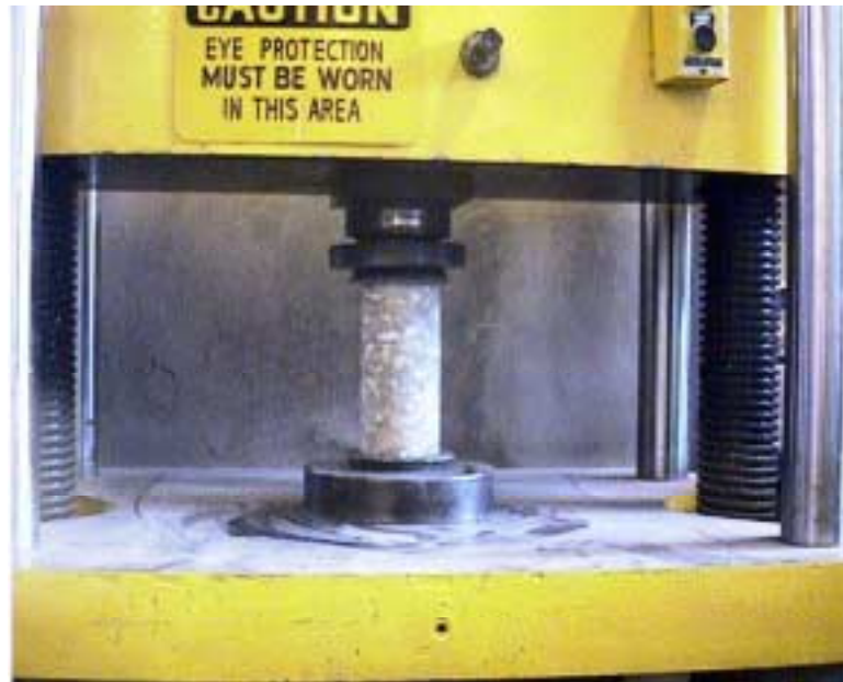
(a) Uniaxial compression test setup
