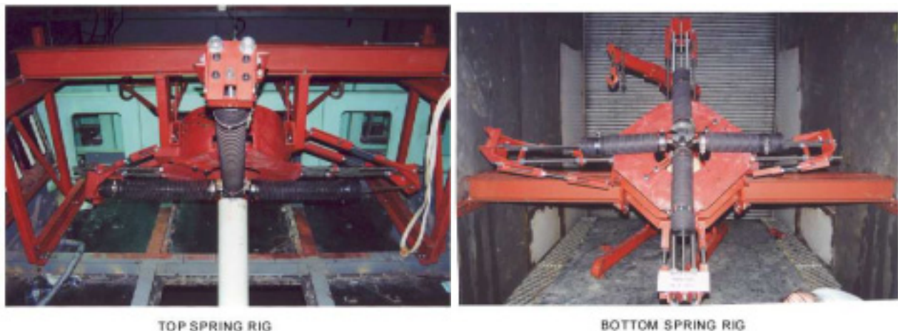
Figure 38: Cable supporting rig.
