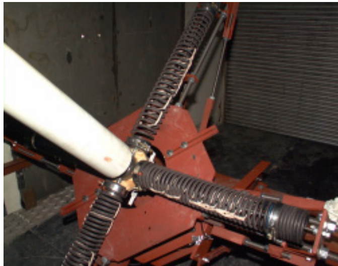
Figure 44: Elastic bands on the spring coils.
