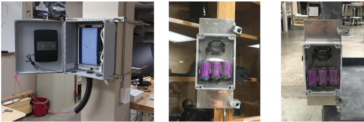
Figure 5. System laboratory setup including a data acquisition system attached to a column (left), sensor node attached to a cabinet (middle), and sensor node attached to a movable cart (right)
