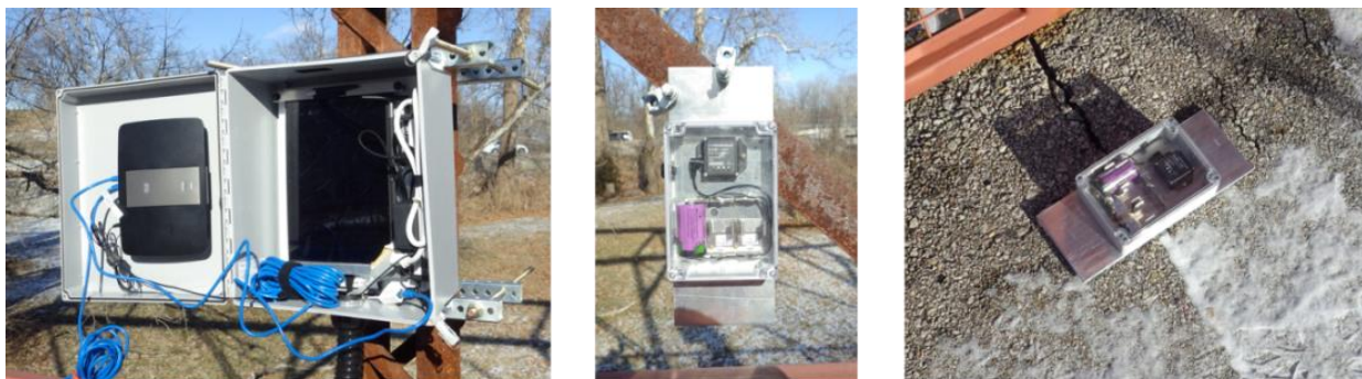
Figure 8. Attachment of the data acquisition system (left), attachment of sensor to a tension tie (middle), and placement of sensor on the deck (right) during field implementation test
