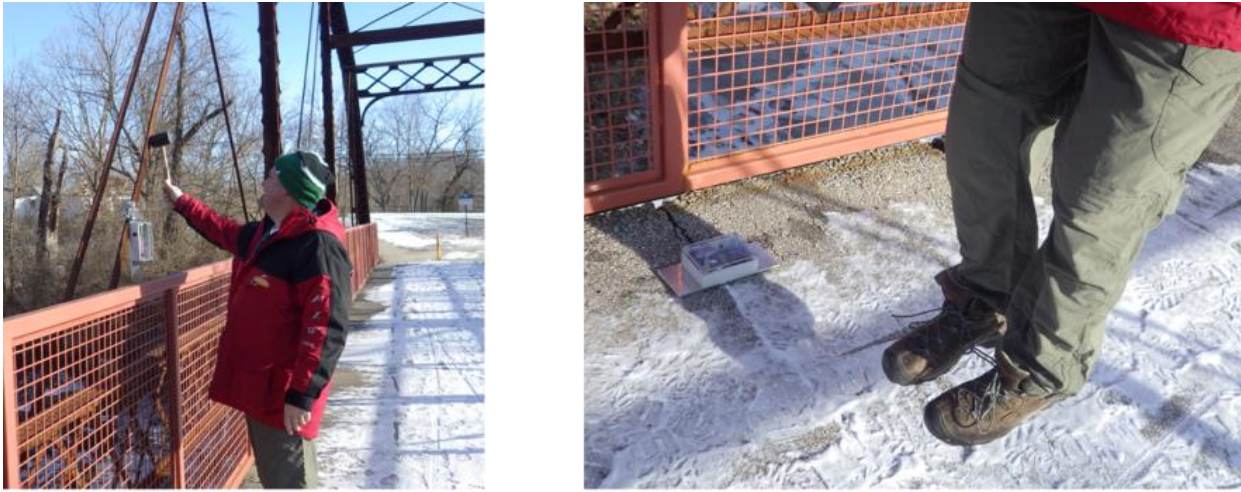
Figure 9. Impact on a tension tie via rubber mallet (left) and impact on the deck by jumping (right) during field implementation testing
