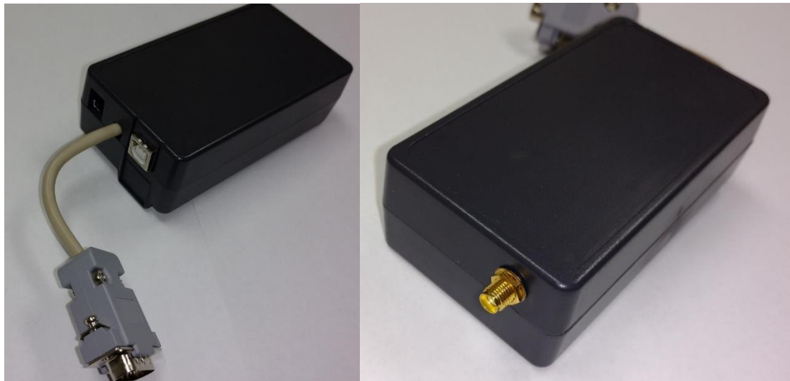
Figure 2. GPS logger (inside plastic housing case), front and back.
