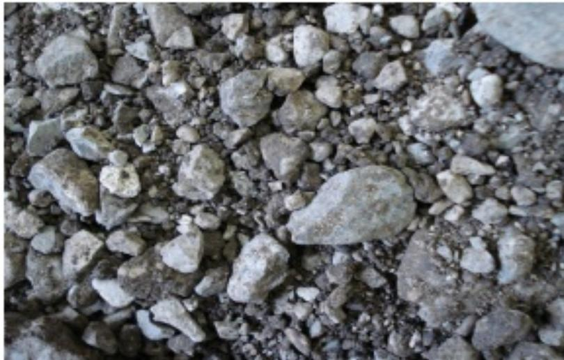
**Figure D-1. Reclaimed asphalt pavement (RAP)**
