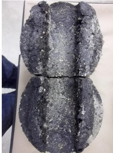
**Figure D-23. Moisture sensitivity of virgin mixture specimen**
