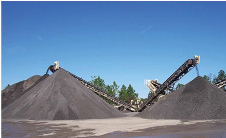
**Figure D-5. Fractionated RAP stockpiles**
