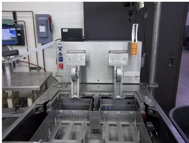
**Figure D-13. Hamburg Wheel Tracking device**
