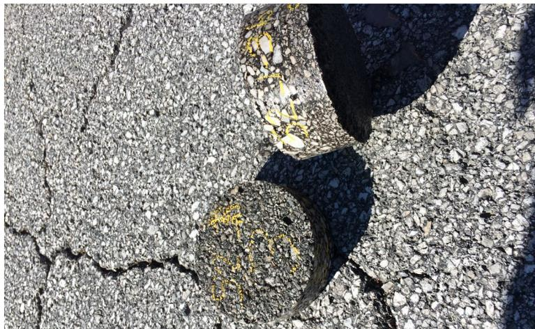
**Figure A-4. Field cores from MO52\_1**
