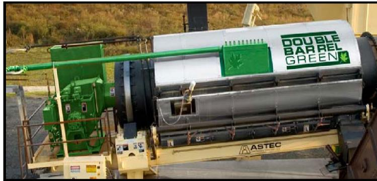
**Figure D-9. Astec double barrel green foaming drum**
