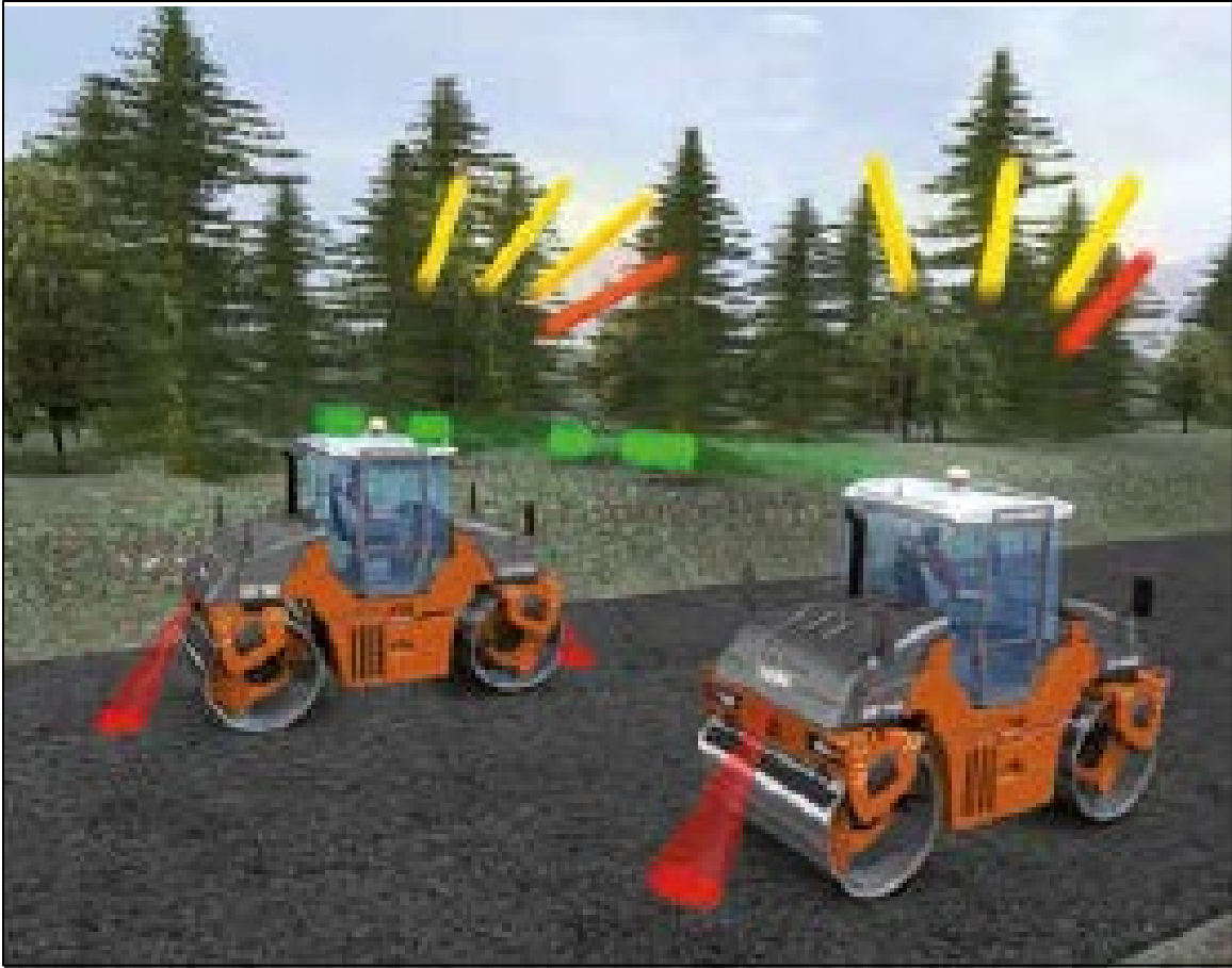
Figure 11: HAMM HCQ Intelligent Compaction System in Echelon Mode with Wi-Fi Connection
