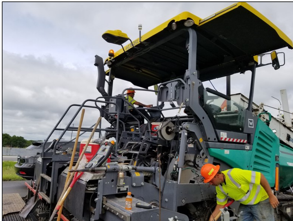
Figure 14: Vogele RoadScan PMTPS Mounted on a Vogele Paver On-site (HWY 61/24 Project)
