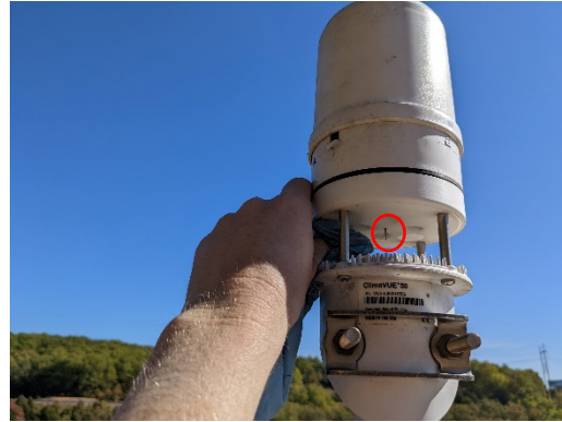
Figure 4: Funnel (rain gauge) at top of weather station. Wipe out gently and remove any leaves. Clear out the temperature sensor area at the base of the weather station. Do not hit the temperature sensor (circled in red in the photo on the right).
