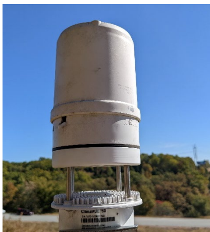
Figure 3: Weather Station at Upper Enclosure. Note cable running from logger to weather station.
