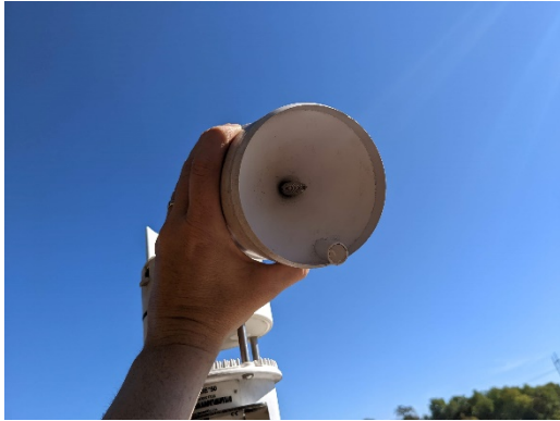
Figure 4: Funnel (rain gauge) at top of weather station. Wipe out gently and remove any leaves. Clear out the temperature sensor area at the base of the weather station. Do not hit the temperature sensor (circled in red in the photo on the right).
