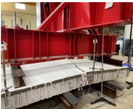
Figure 1: Flexural testing of composite slabs repaired with thin bonded UHPC overlay
