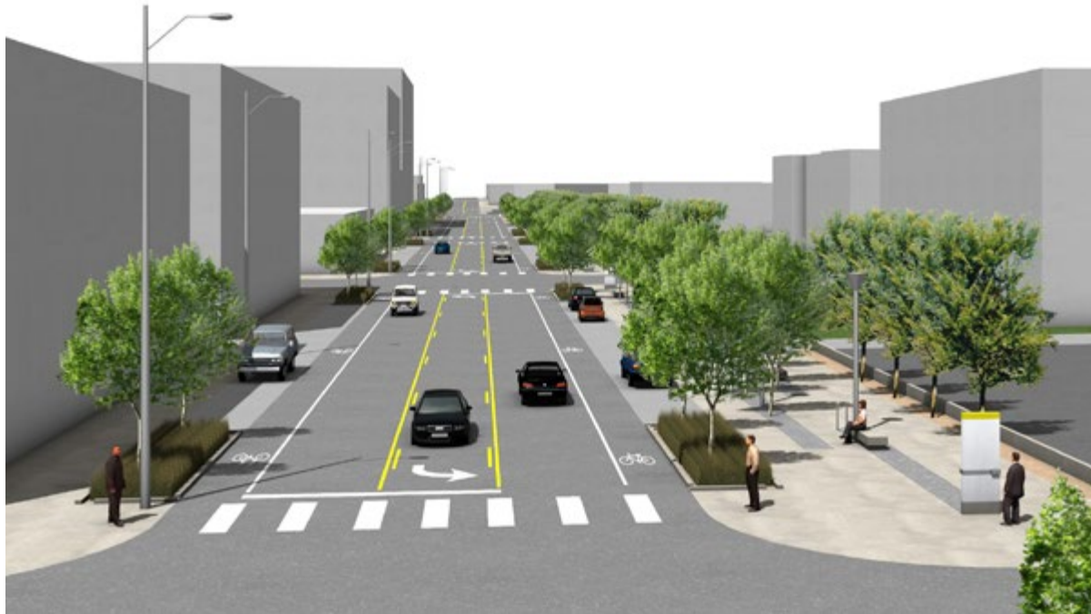
Figure 7-3 Example of a Drawing of a Road Diet (Source: BikeWalkKC)
