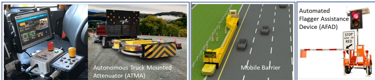
Figure 2.5 Autonomous Truck Mounted Attenuator (ATMA) Mobile Barrier, and Automated Flagger Assistance Device (AFAD)
