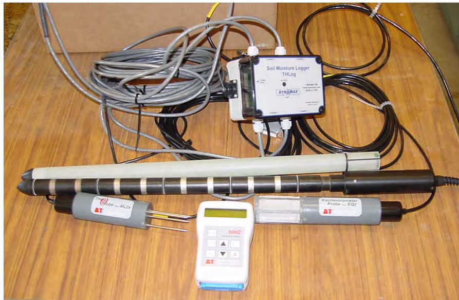
Figure 5.11 Instrumentation used to monitor soil water conditions at the I435-Kansas City site and other sites: ThetaProbe ® ML2x (bottom left), Equitensiometer ® EQ2 (bottom right), THLog ® data logger (top center), Profile Probe ® PR1/6 and access tube (center), and HH2 readout unit (lower center).
