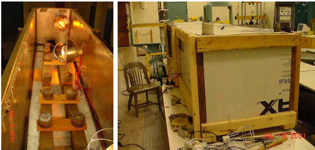
Figure 5.3 Photographs of temperature controlled box utilized for curing the adhesive used to attach strain gages to recycled plastic members.
