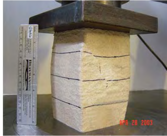
(a) Typical failure mode for compression molded specimens from manufacturer A.
