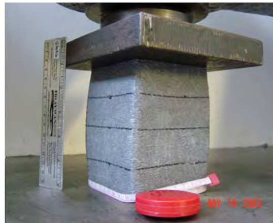
(b) Typical failure mode for extruded products from manufacturers B and C.
