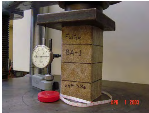
Figure 3.2 Setup for uniaxial compression tests.
