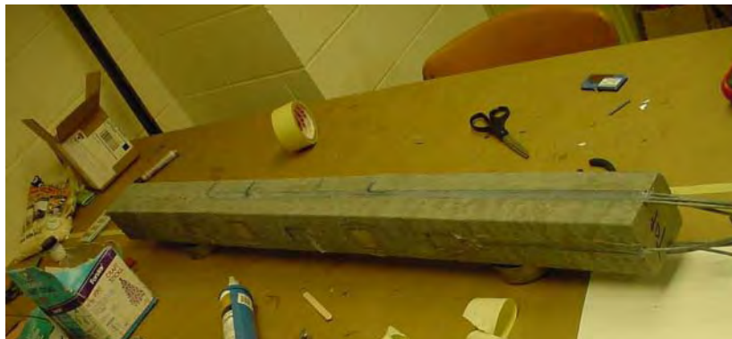
Figure 5.1 Instrumentation used to monitor loads in recycled plastic reinforcing members: (a) schematic of instrumented member and (b) photograph of an instrumented test member.
