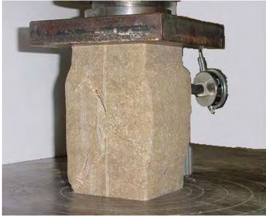
(a) Typical failure mode for compression molded specimens from manufacturer A.
