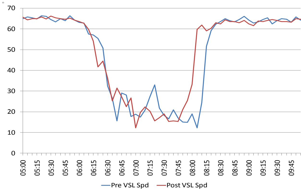
Figure S2.12.1. Comparison of Pre (Oct 14 th , 07) and Post-VSL (Oct 16 th , 08) Speed data for 3D
